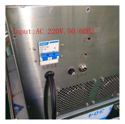
Turn on the work switch, Adjust the output voltage.
