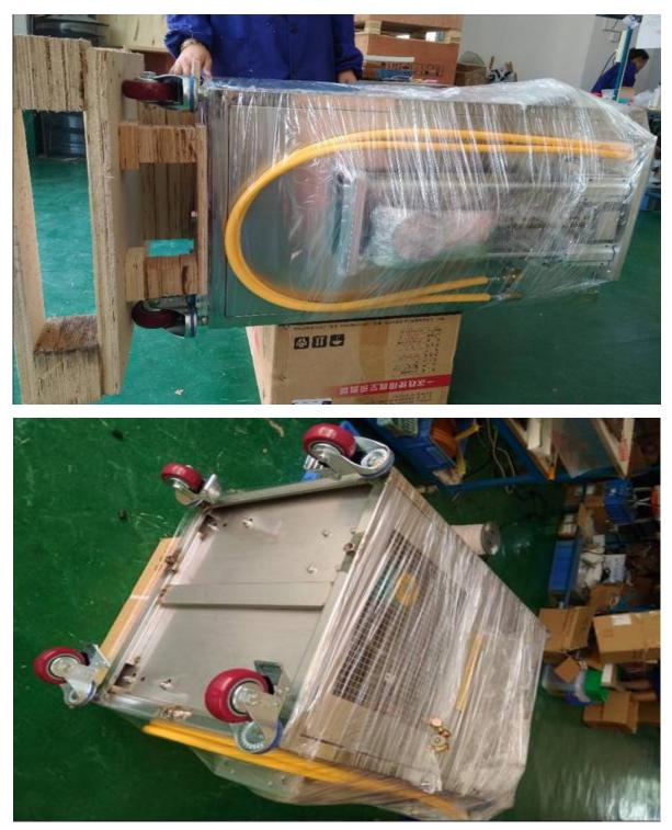
Remove the protective film and tack out the tools and hanging board from the lifting platform. Then remove the remaining protective film on the lifting platform.Fix the hanging board on the lifting platform and tighten with the four M8\*25 hex screws in the kit.Fix the black handle onto the lifting platform with the hexagon socket head cap screw.
